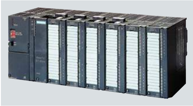
SIMATIC ET 200M with power supply
