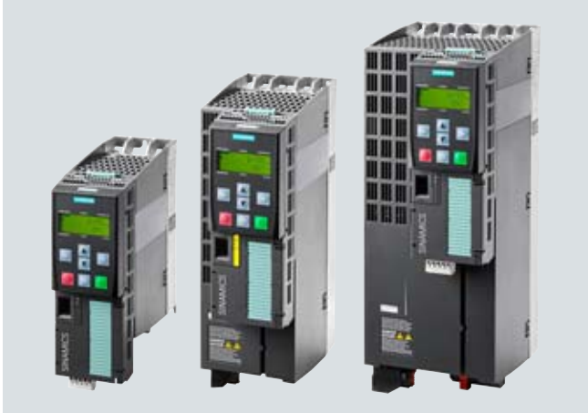
SINAMICS G120P in degree of protection IP20 standard variant, frame sizes FSA to FSC comprising PM230 Power Module, CU230P-2 HVAC Control Unit and mounted Basic Operator Panel BOP-2
