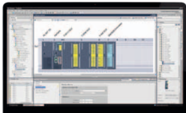
Device View S7-300 rack with safety IO
