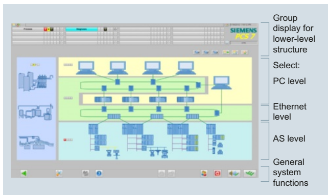
Plant overview with symbol displays for components
